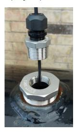
The 1" NPT adapter is tightened into the 2" adapter and the pressure sensor lead fed into the tank until the bottom of the sensor is positioned approximately 50mm above the bottom of the tank. The cable grip is tightened (torque 1-8 to 2Nm) around the cable to hold it in position.
