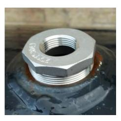
The Pressure logger sensor comes fitted with a 1" NPT adapter and a ½" NPT cord grip cable adapter. The pressure sensor fits through the 1" opening and is placed into the tank.
