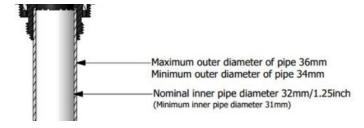
The pipe should be cleanly cut to length. The length required should be measured from the top of the tank (where the sensor is to be mounted) to that of the fuel outlet point (as shown).
